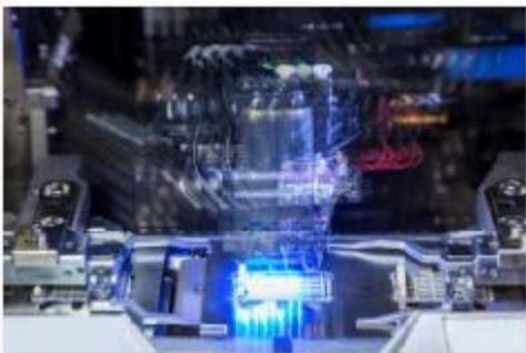
The gold wire bonder, which is used for the electrical contacting of the UV LED chips, is at the heart of the production process. It produces very robust connections, exceeding even industrial standards.
